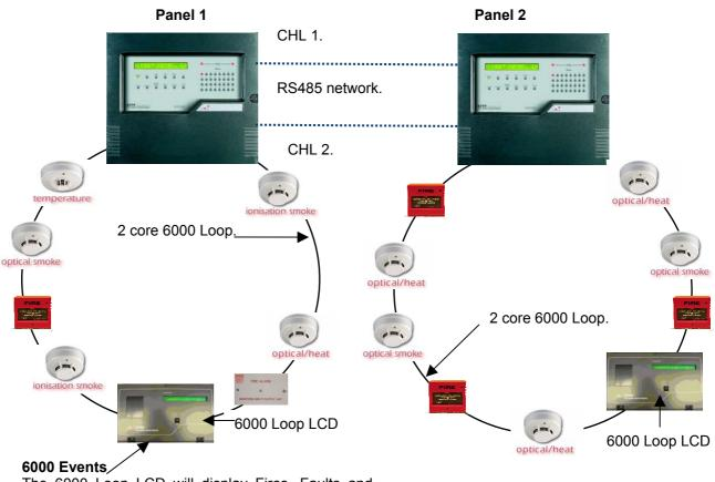
The 6000 Loop LCD will display Fires, Faults and Isolations for all events on the 6300 network. The LCDs are configured for displaying all events as factory default settings. An option for filtering these events will be available in future software.
