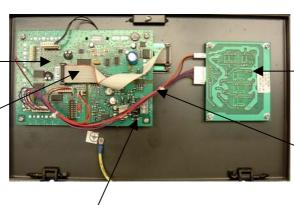
LED display PCB. PCB for the three LED indicators
